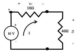
Note that the first polarity encountered of the voltage source is "-", which is reflected in the equation. The third step is applying Ohm's law for each element voltage using the mesh current I, and the specific resistor, substituting  $I^*R_x$  for each V in the equation.
