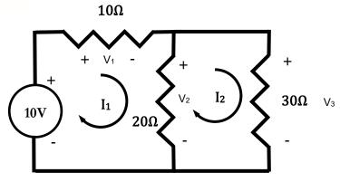
First, assign voltage variable names and polarities to each circuit element. Then identify the currents in each mesh and assign each current a variable name. Next, starting at a node in the desired mesh, follow each current around the mesh and note the variable name and polarity. Lastly, apply Ohm's Law to each element.
